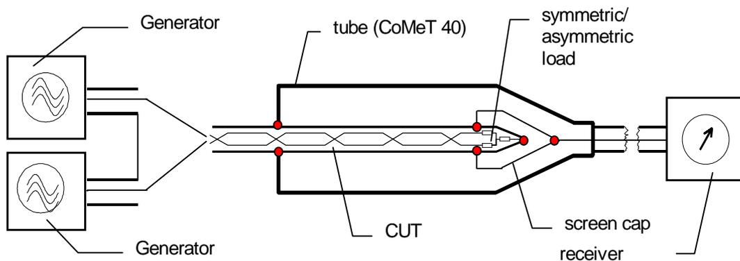
**Fig. 4 – Principle set-up to measure the coupling attenuation of screened balanced cables**
