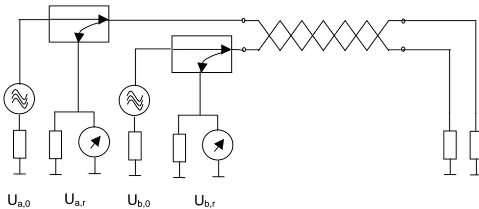
**Fig. 2 – Test set-up for impedance and return loss measurements**
