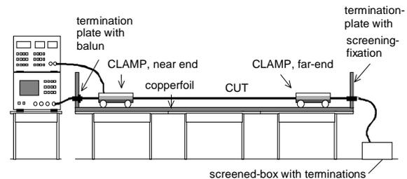
Fig. 9: injection clamp set-up
