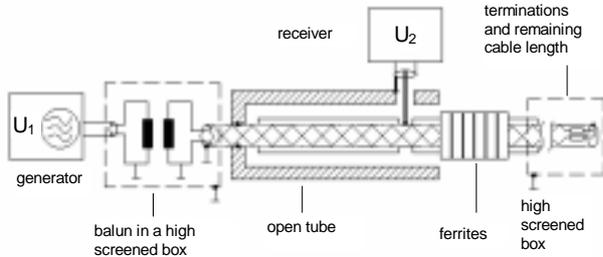
Fig. 10: Triaxial set-up to measure the coupling attenuation
