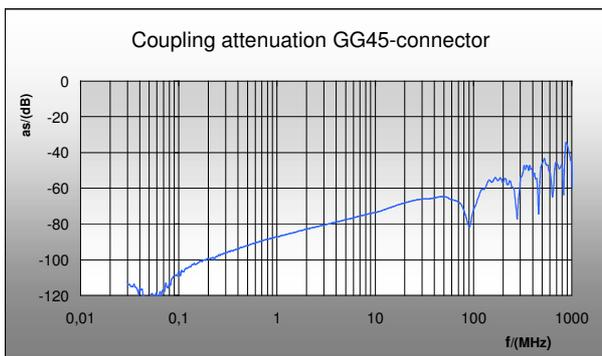
Figure 7 – Measurement of the coupling attenuation of a GG45 connector
