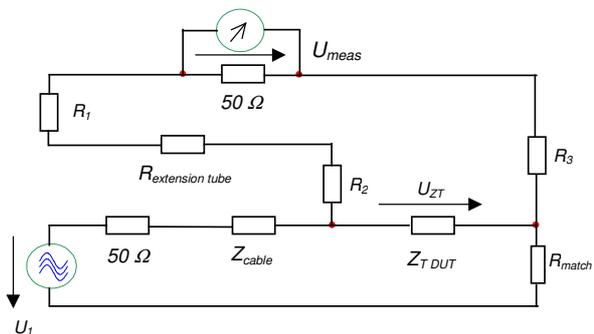
Figure 9 – Equivalent circuit of the test set-up with contact resistances
