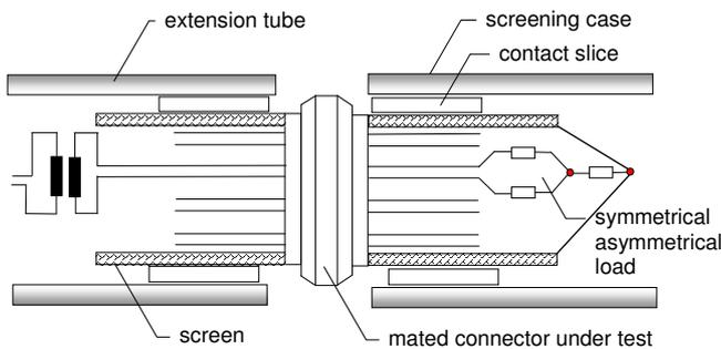
**Figure 4b – Principle preparation of balanced or multiconductor connectors for coupling attenuation**
