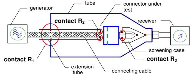
Figure 8 – Contact resistances of the test set-up
