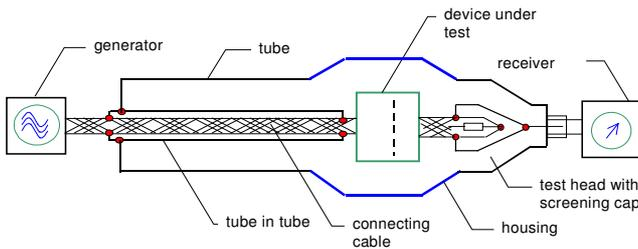
**Figure 10 – Principle test set-up for measuring the Screening attenuation of connecting hardware with the Tube in tube procedure**
