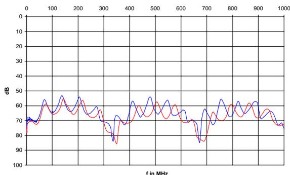
Fig. 11b: screening attenuation of RG 58 measured with the common and modified triaxial set-up; linear frequency scale
