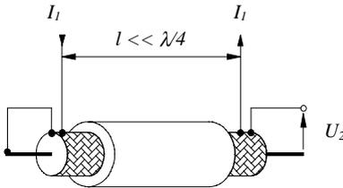
Fig. 2: Definition of transfer impedance
