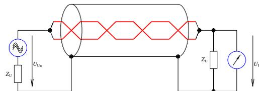
Fig. 5b: Common mode of a screened pair (STP)
