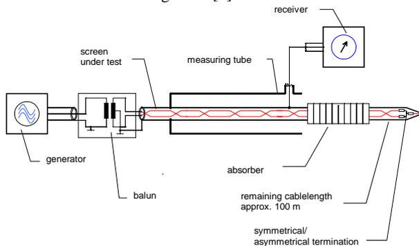
Fig. 10: Set up to measure the coupling attenuation in the modified triaxial set-up.
