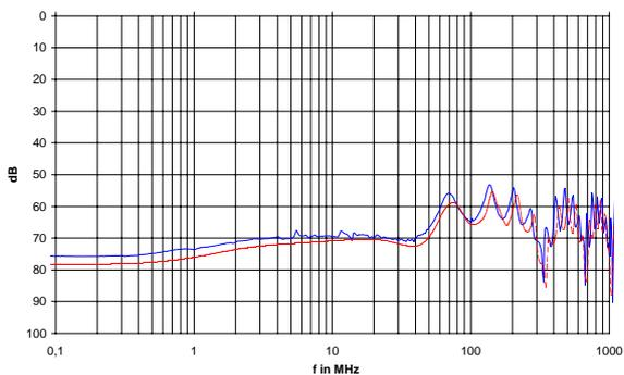
Fig. 11a: screening attenuation of RG 58 measured with the common and modified triaxial set-up; logarithmic frequency scale
