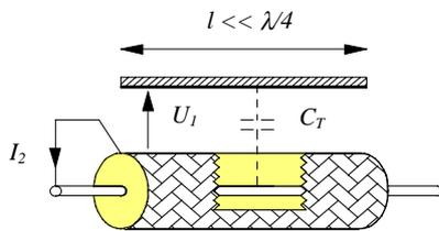
Fig. 3: Definition of coupling admittance
