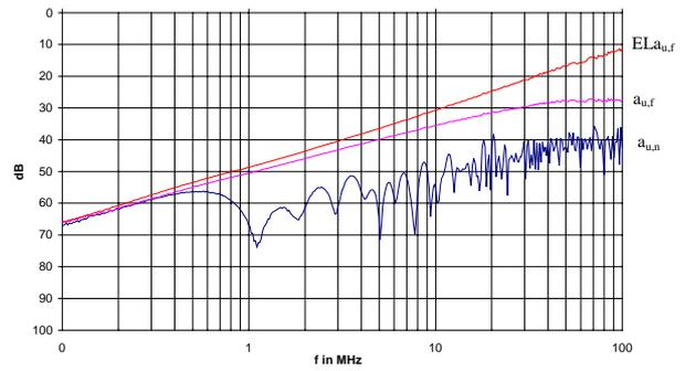
Fig. 7: Unbalance attenuation of Twinax 105 Ohm
