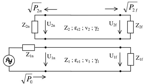
Fig. 0: Equivalent circuit for general coupling transfer function
