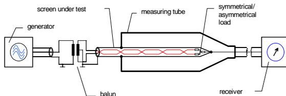
Fig. 9: Set up to measure the coupling attenuation in the triaxial set-up.
