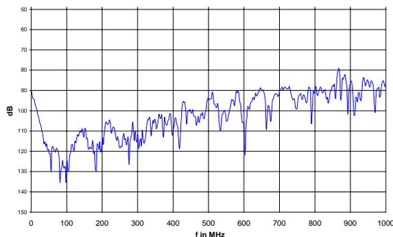
Fig. 12b coupling attenuation of a common Cat 6 cable, coupling length 207 cm; logarithmic frequency scale.
