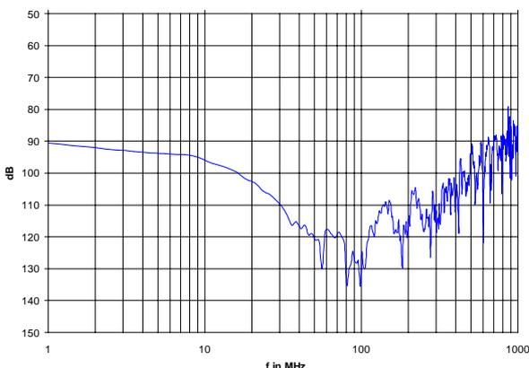
Fig. 12a: coupling attenuation of a common Cat 6 cable, coupling length 207 cm; logarithmic frequency scale.
