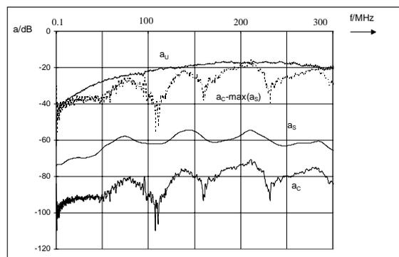
Fig. 13: Curves of unbalance, screening attenuation, coupling attenuation and calculated unbalance of a screened twisted pair (Twinax 105).
