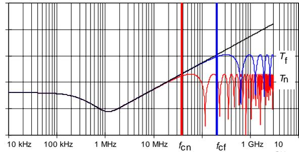
Fig. 4: calculated coupling transfer function ( $l = 1$  m;  $\epsilon_{r1} = 2,3$ ;  $\epsilon_{r2} = 1$ ;  $Z_F=0$ )
