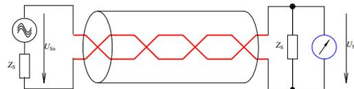
Fig. 5a: Differential mode of a screened pair (STP)
