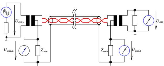
Fig. 6: Measuring set-up for unbalance attenuation
