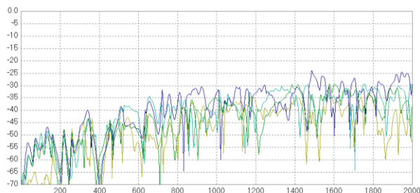
Figure 17b – Far end coupling attenuation of an unscreened Cat5e acc. to figure 13, Ssd21, lin
