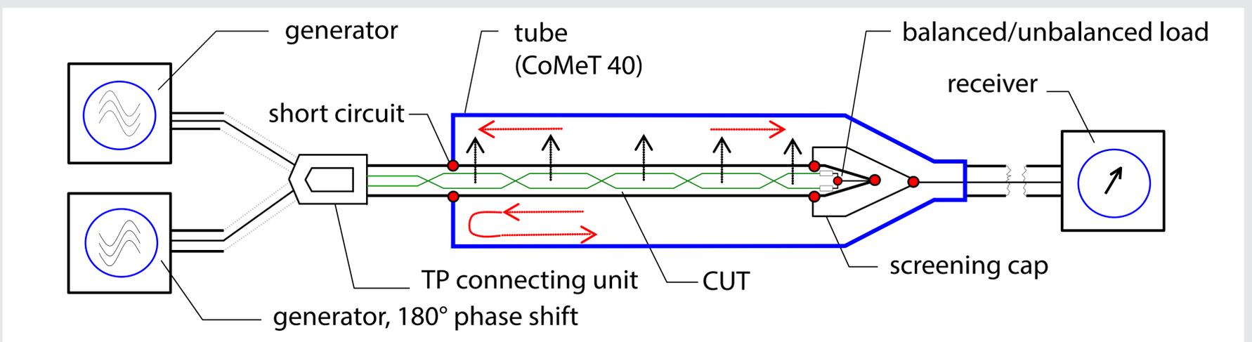
IEC 62153-4-9 Ed.2: Coupling Attenuation  $a_c$  – Triaxial Method
