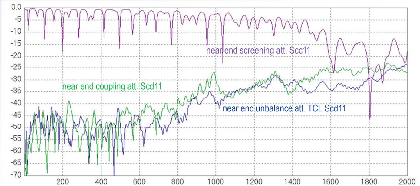
**near end coupling attenuation of a single unscreened balanced pair = TCL !**
