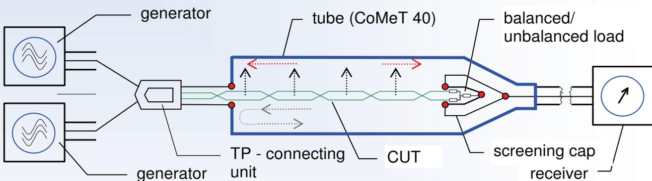
set-up for the far end screening attenuation (Scs21) and the far end coupling attenuation (Ssd21) measurement of an unscreened pair.
