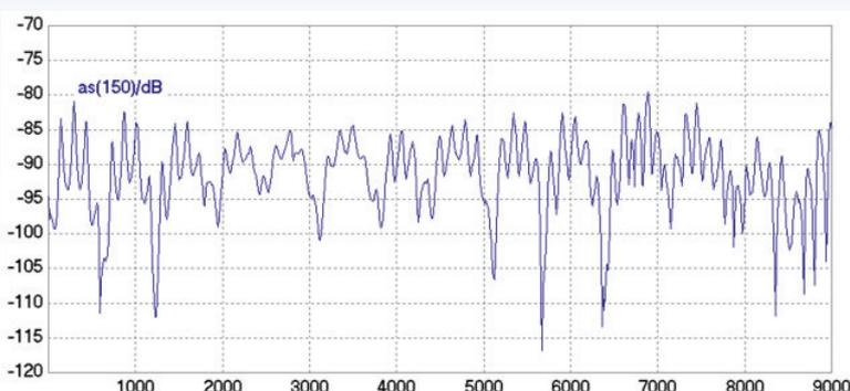
*Screening attenuation of a RG 214 up to 9 GHz in Triaxial cell with magnetic absorber*
