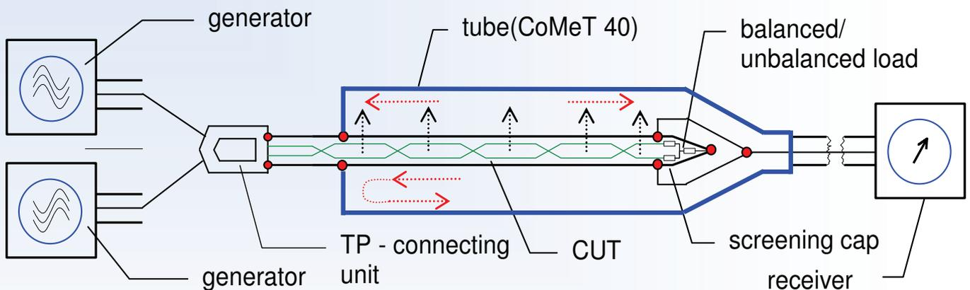
The principle for coupling attenuation measurement on screened balanced cables is the same than the basic triaxial procedure with a generator (respectively 2 generators) a receiver and a short circuit at near end.
