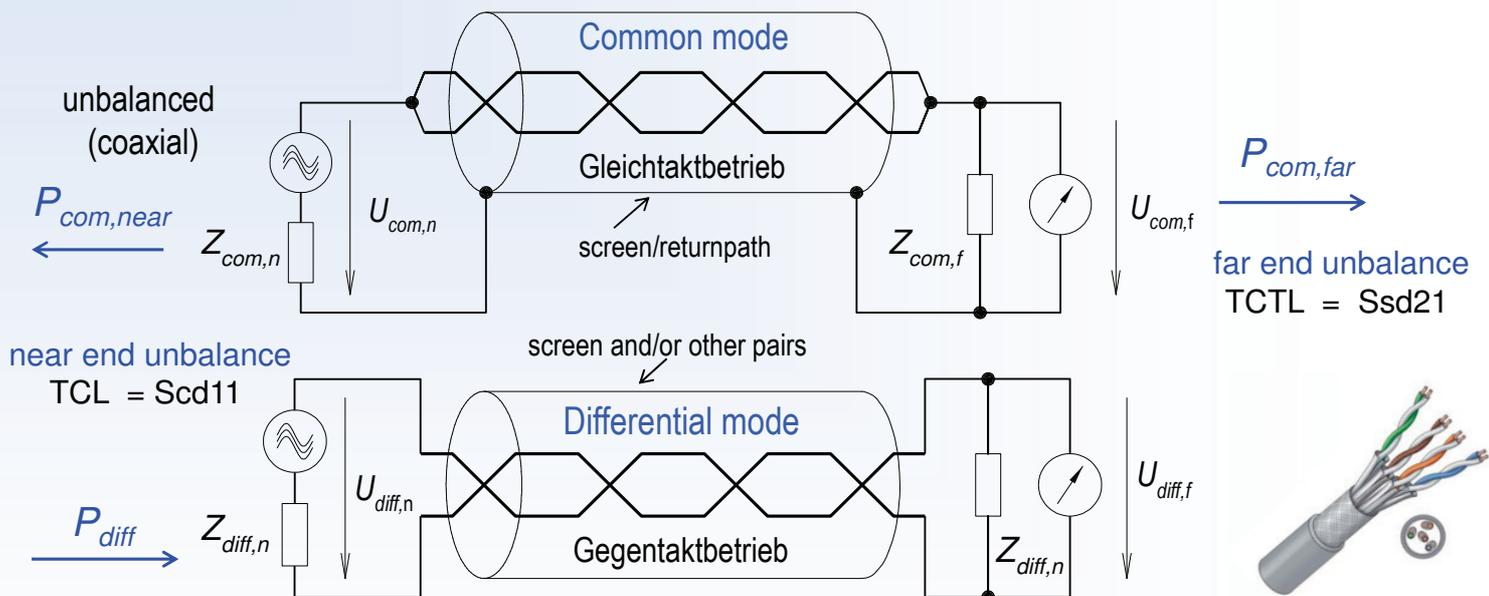
Balanced cables can be operated in the common mode as well as in the differential mode.
