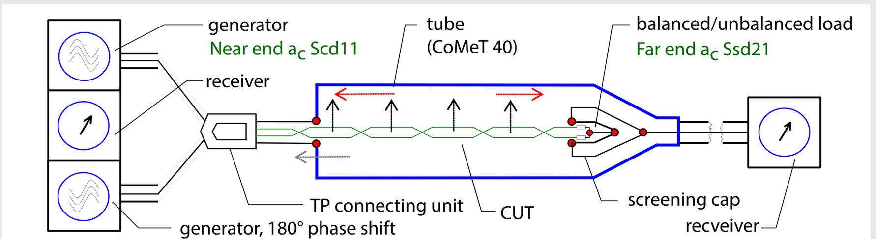
IEC 62153-4-9 Ed.2 Amd.1: Coupling Attenuation  $a_c$  of Unscreened Balanced Pairs
