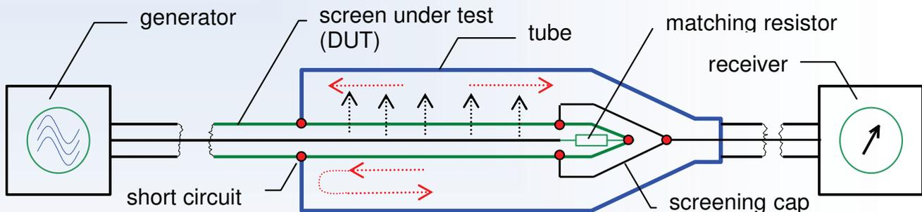
The triaxial set-up consists of the DUT in the middle of the tube, the generator and the receiver included in a modern VNA, the matching resistor at far end and the short circuit at near end. The DUT is fed by the generator. Due to the weak screen, energy is coupling into the outer system respectively in the tube and a wave is travelling in both directions first.
