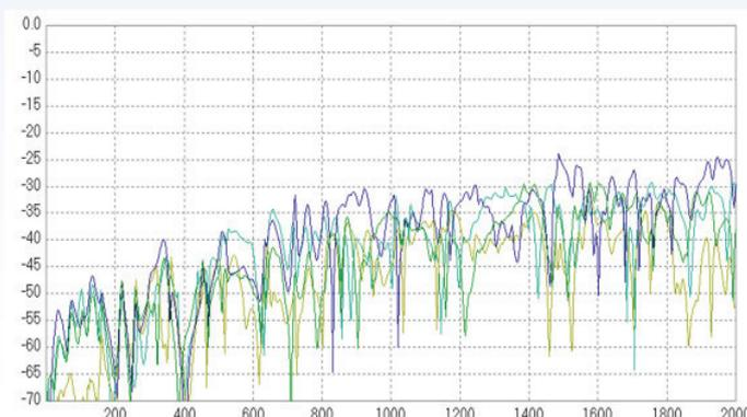
far end coupling attenuation of an unscreened Cat5e (Ssd21)
