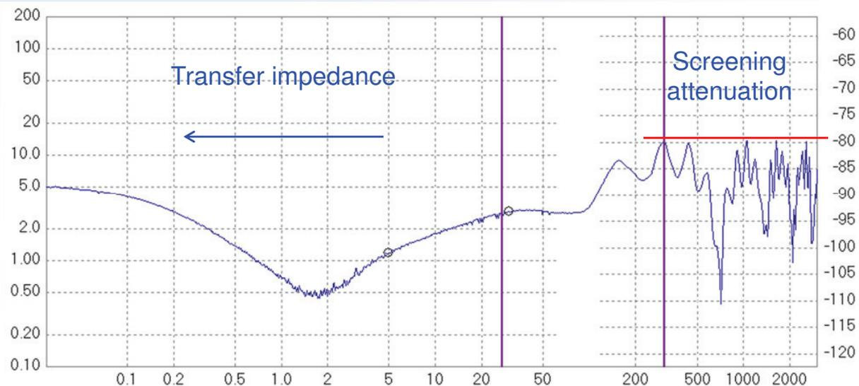
Breitenbach realized, that the max. values of the resonances of the triaxial procedure at higher frequencies could be used as measure of the **Screening attenuation** up to and above 3 GHz.
