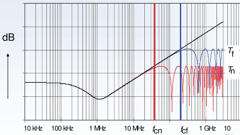
The Coupling Transfer Function  $T_{nf}$  results from the multiplication of the equivalent Transfer impedance  $Z_{TE}$  and the **Summing function**  $S_{nf}$
