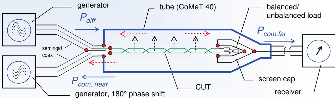
This figure shows the principle set-up for **balanced unscreened pairs**. The principle is the same than the balunless procedure for screened balanced cables. Since there is no screen on the unscreened pair, there is no short circuit at the near end as in the basic triaxial set-up;
