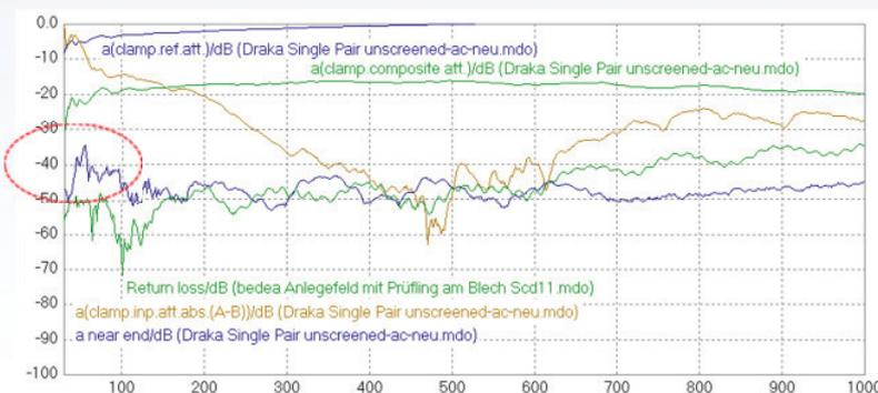
**Coupling attenuation** of an unshielded balanced pair with absorbing clamp MDS 21
