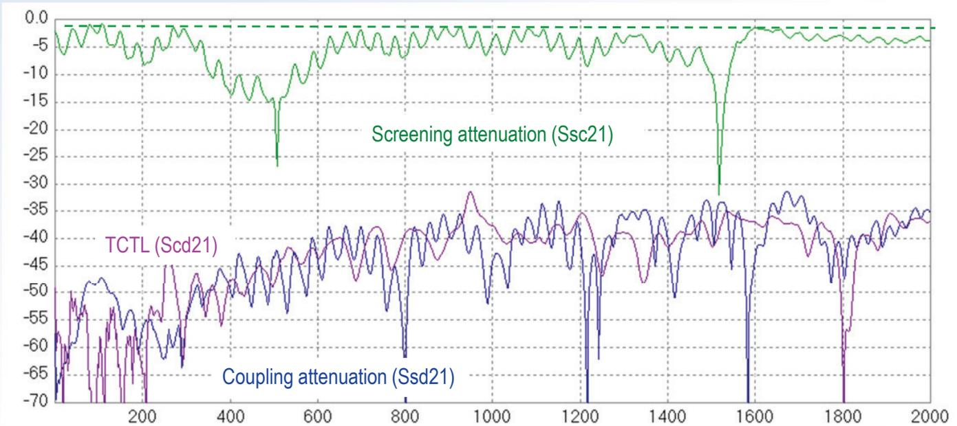
**far end screening attenuation of a single unscreened balanced pair = nearly zero !**
