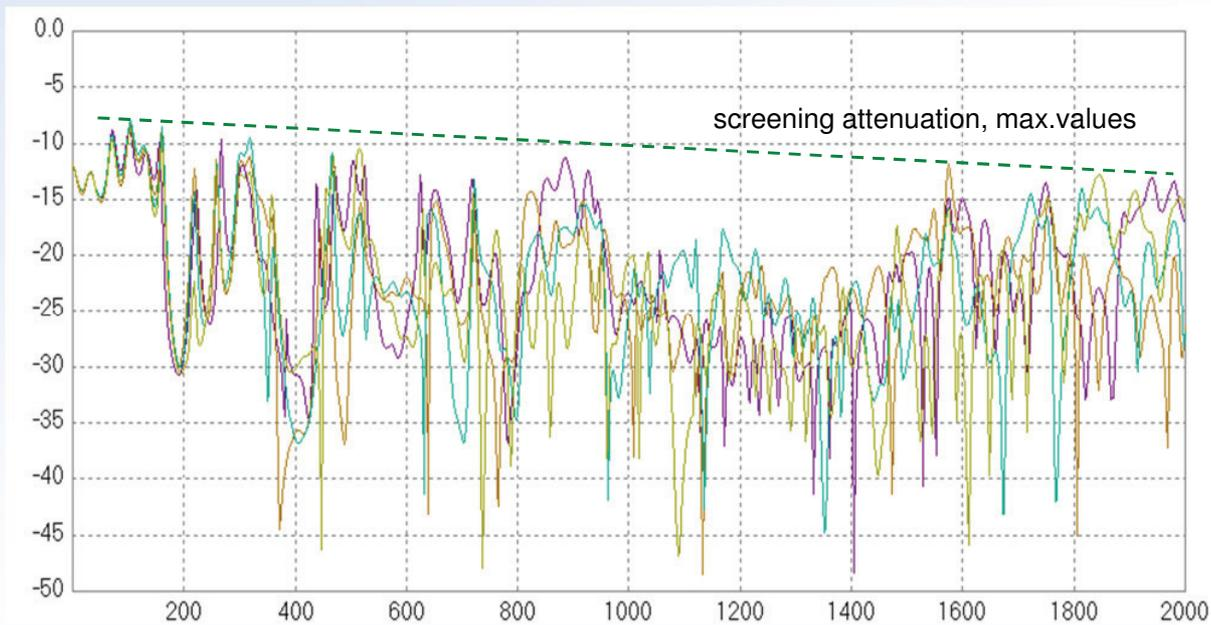
The measured screening attenuation (Ssc21) of about 8 to 12 dB of the unscreened pairs can be explained by the remaining pairs which acts as “inner screen”.
