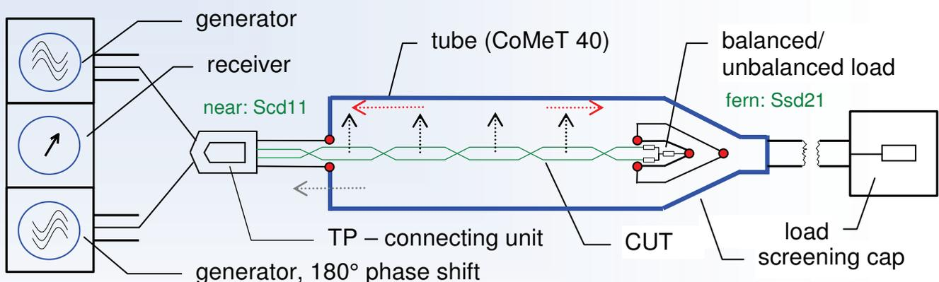
This figure shows the configuration for **near end coupling attenuation** measurement. The back travelling energy at the near end as shown above is considered as the near end coupling attenuation.
