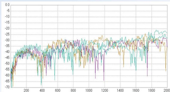
far end unbalance attenuation of an unscreened Cat5e (Scd21)
