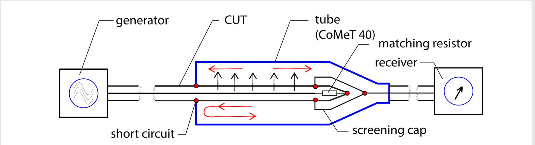
IEC 62153-4-3/-4 Ed.2: Transfer Impedance  $Z_T$  & Screening Attenuation  $a_s$
