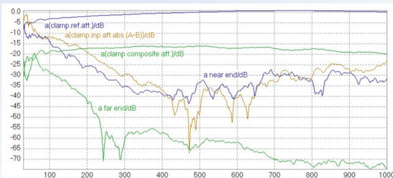
**Screening attenuation** of an unshielded balanced pair with absorbing clamp MDS 21
