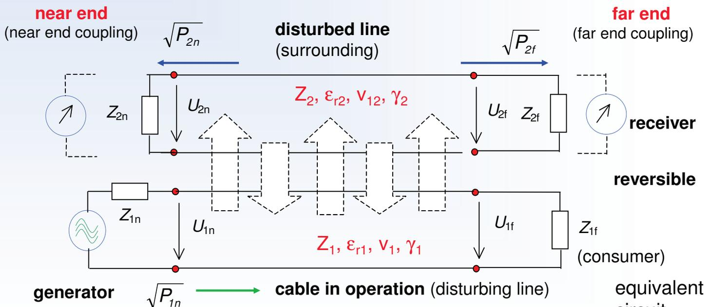
Char. impedance **Z**, dielectric constant  $\epsilon_r$ , velocity of propagation **v**, propagation constant  $\gamma = \alpha + j\beta$
