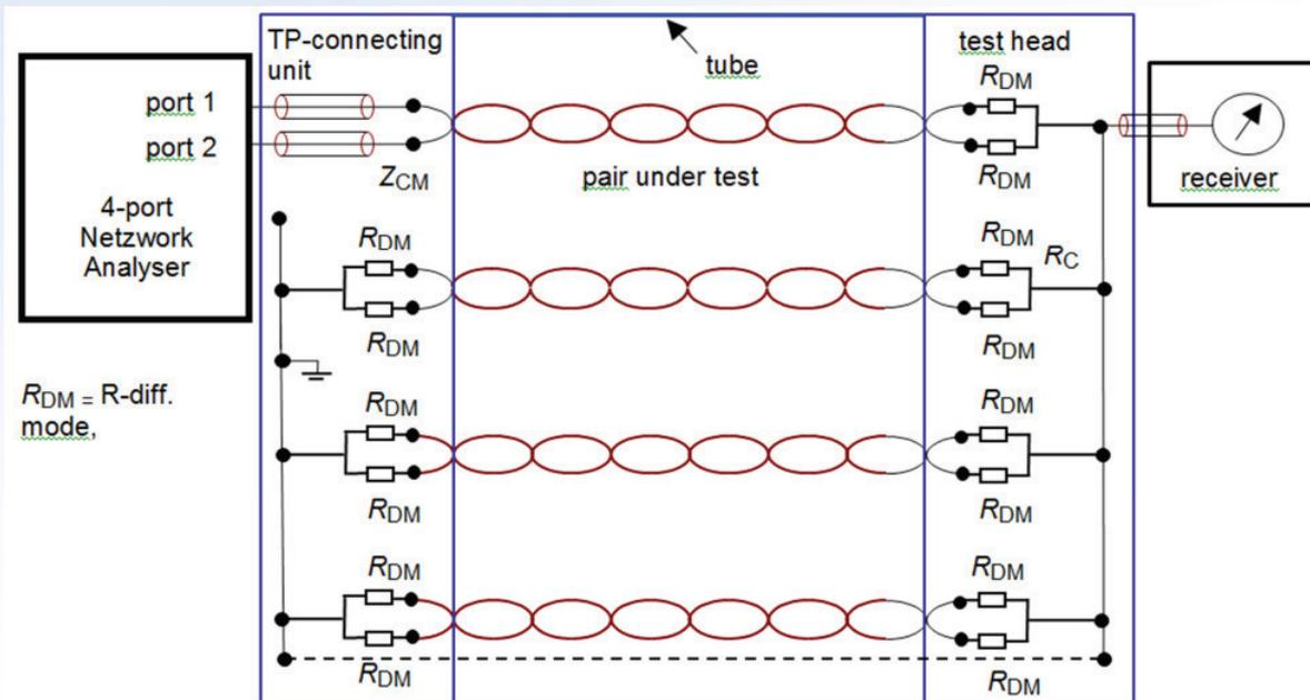
The pairs not under test are grounded by a resistor network 50/50/0. They act as an inner screen
