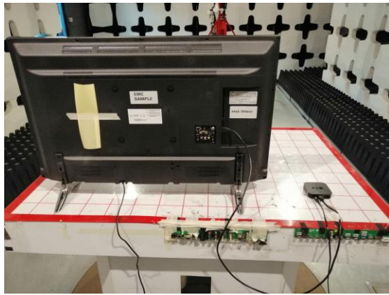
Figure 10. Test configuration for radiated emission measurement (Vestel EMC lab)
