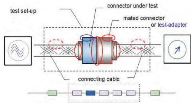
**Fig. 9 — Influencing variables when measuring the EMC of a connector.**
