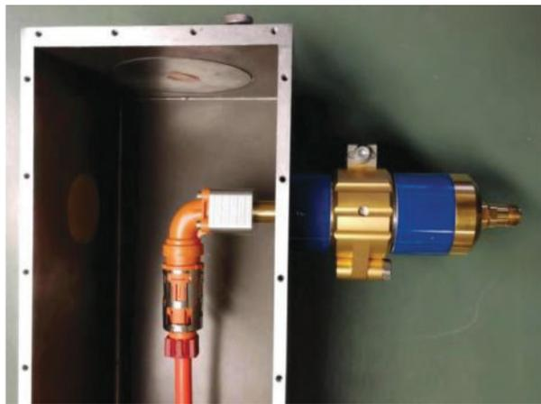
**Fig. 12** — Angled HV connector in triaxial cell.
