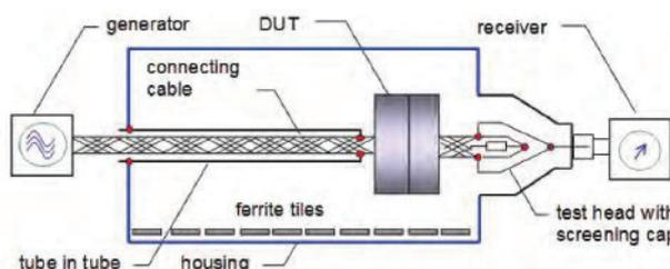
Fig. 3 — Principle of the Triaxial cell with tube in tube and ferrite tiles as absorber.
