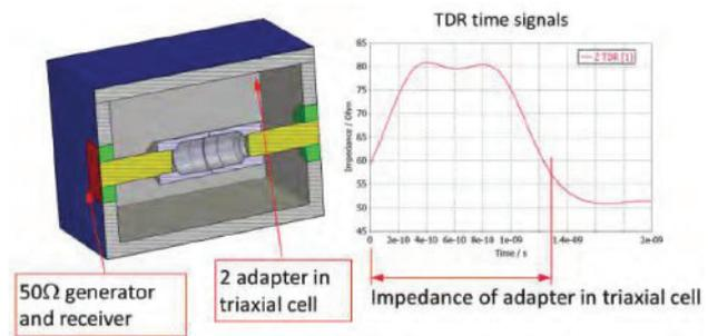
**Fig. 10 — Simulation of a test adapter in a triaxial cell .**
