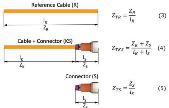
Fig. 7 — Delta transfer impedance.
