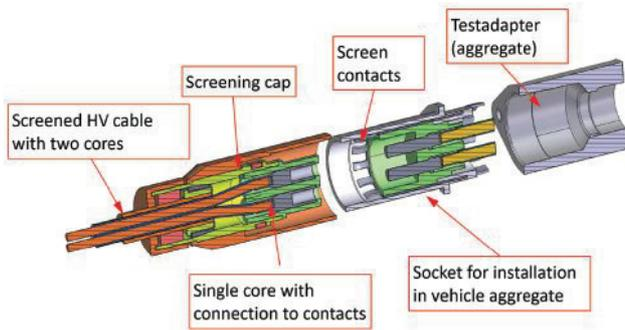
Fig. 5 — Basic replication of a HV connector and installation in the triaxial cell.
