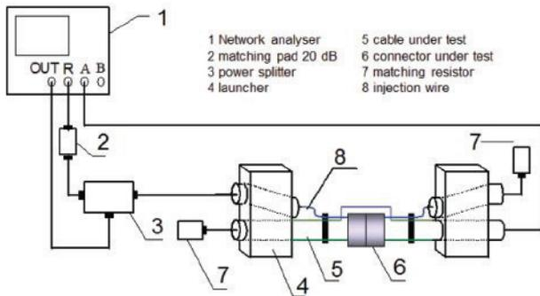
Fig. 4 — Principle of the line injection procedure.
