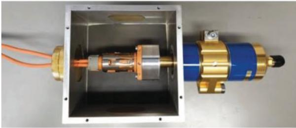
**Fig. 11** — Straight HV connector in triaxial cell.
