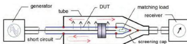
Fig. 2 — Basic triaxial test procedure.
