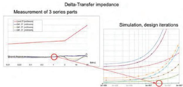
**Fig. 13** — Transfer impedance, comparison of measurement (left) and simulation (right).
