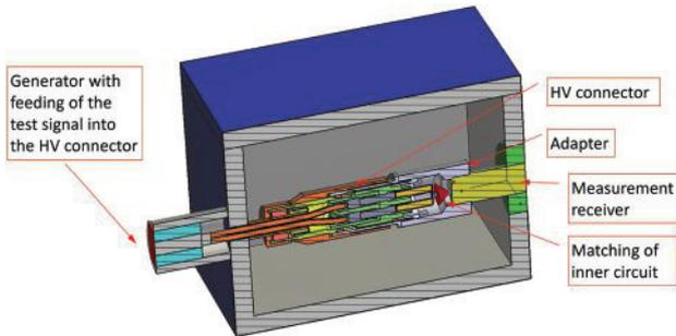
Fig. 6 — Triaxial cell with HV connector.
