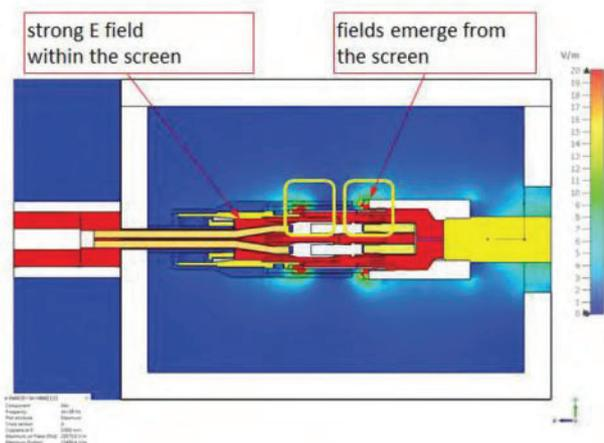
**Fig. 8 — Analysis of the weak points of a HV connector due to leaked E-fields.**
