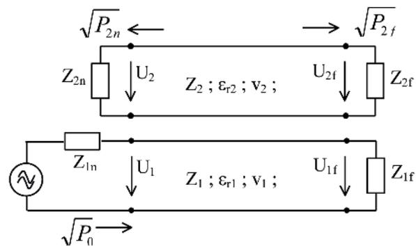
Fig. 1 — Equivalent circuit of the coupling of two lines.
