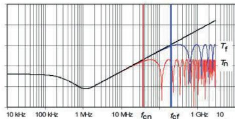
Fig. 5 — Calculated coupling transfer function, ( $l = 1 \text{ m}$ ;  $\epsilon_{r1} = 2,3$ ;  $\epsilon_{r2} = 1$ ;  $Z_F=0$ ).
