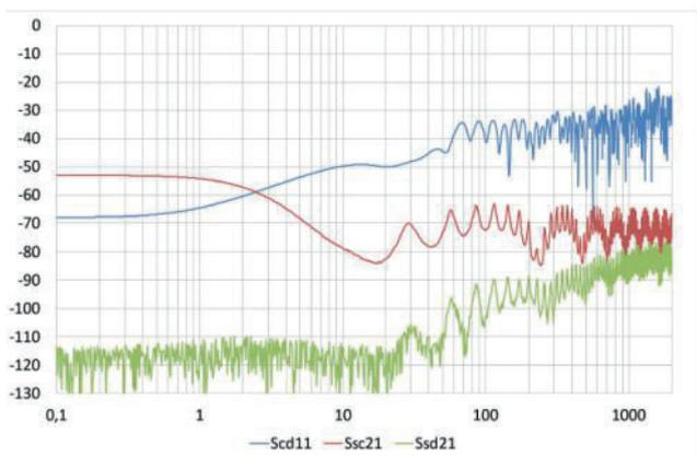
Fig. 10 — Calculated near unbalance attenuation (Scd11) as well as screening attenuation (Ssc21) and coupling attenuation (Ssd21) of a shielded single-pair AWG23/1 cable, coupling length 5 m, raw values.
