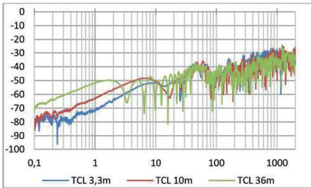
Fig. 14 — Near end unbalance attenuation TCL at different length of a screened single pair cable AWG23/1.
