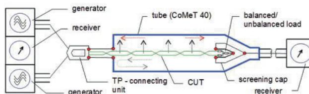
Fig. 13 — Measurement of the coupling attenuation of unshielded cables according to IEC 62153-4-9 Amd1.
