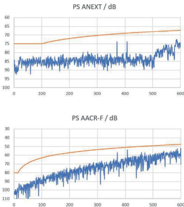
**Fig. 19 — Alien-Crosstalk measurement “6 around 1” on a highly shielded single-pair AWG 22/7 cable, measuring length 100 m.**
