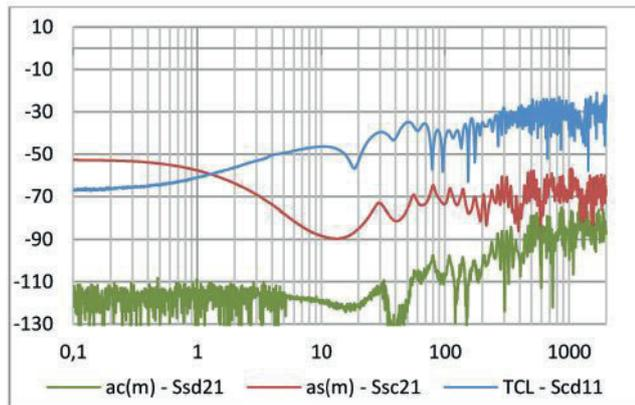
Fig. 16 — Near unbalance attenuation as well as screening attenuation and coupling attenuation of a single-pair shielded AWG23/1 cable, measuring length 5 m, raw values.
