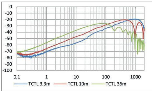
Fig. 15 — Far end unbalance attenuation EL TCTL at different length of a screened single pair cable AWG23/1.
