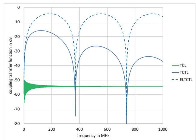
**Fig. 7** — Calculated unbalance TCL, TCTL and ELTCTL of a balanced pair of 50 m, with logarithmic and linear frequency scale.
