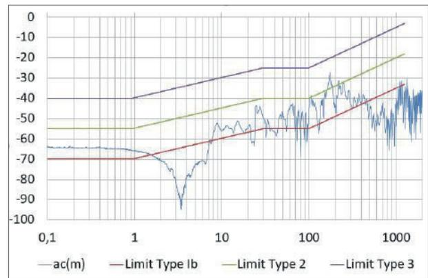
Fig. 17 — LFCA and CA on an unscreened single-pair cable, measuring length 3 m, in comparison with different limit value curves.
