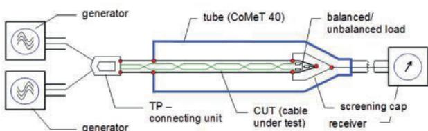
Fig. 12 — Coupling attenuation with virtual balun<sup>25</sup>.
