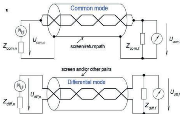
**Fig. 6** — Common and differential mode of a screened twisted pair (STP).
