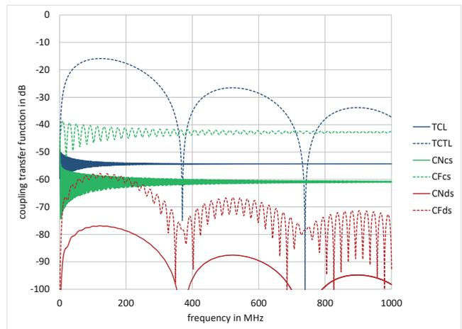
**Fig. 9 — Calculated coupling transfer functions of a shielded pair with systematic coupling and 50 m length, with logarithmic and linear frequency scale.**
