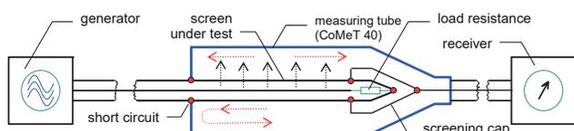
Fig. 11 — Basic triaxial tube procedure.
