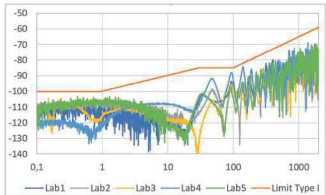
Fig. 18 — LFCA/CA measurements of different laboratories on samples of an AWG 26/7 cable of a production lot.
