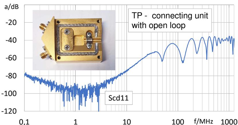
An estimation of the **system mode conversion** can be done by measuring the **Scd11 parameter** of a TP connecting unit with open loop.
