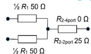
terminating resistors integrated in the test adapter
