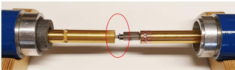
Measuring of **CA/LFCA** of an SPE connector with **tube-in-tube** procedure according to IEC 62153-4-7Ed3 with **ready-made** test adapter
