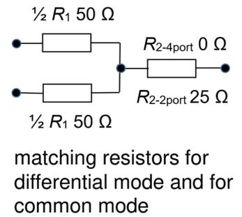
The balanced pair is fed with a 100 Ohm signal by two 50 Ohm generators with 180° phase shift (**virtual balun**). Energy couples from the “differential mode” into the “common mode” (**mode conversion**) and then from the “common mode” into the measuring tube (the outer circuit).
