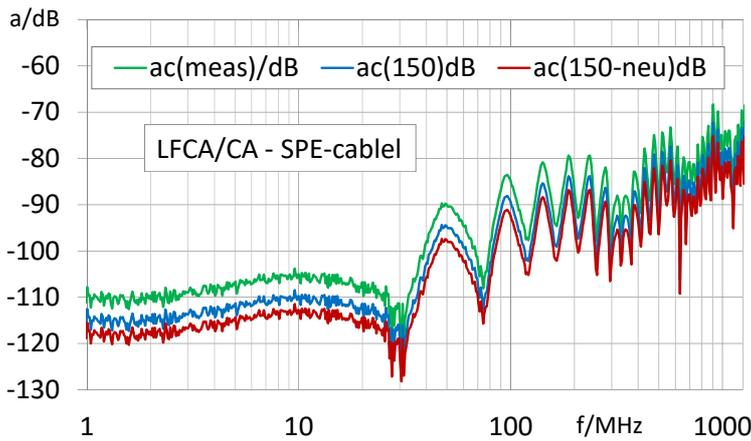
In order to compare triaxial measurements of the coupling attenuation with measurements using absorbing clamps, an arbitrary normalized value of  $Z_S = 150 \Omega$  was introduced in the standards.
