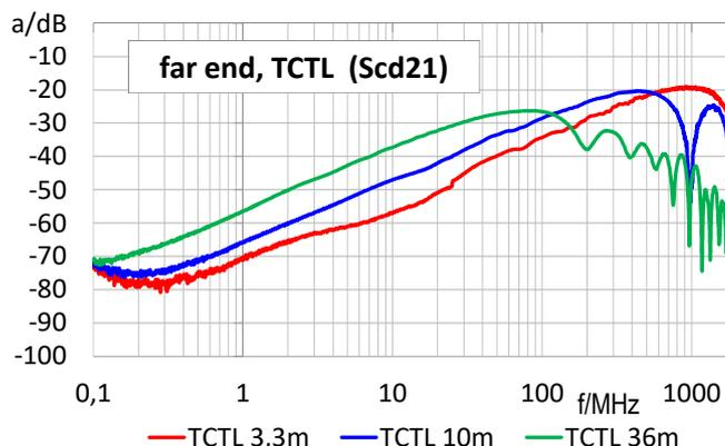
At high frequencies, the unbalance attenuation asymptotically approaches a limit value, (about -25 dB).
