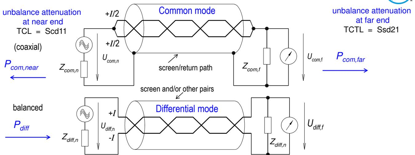
The "Unbalance Attenuation" of a pair describes as logarithmic ratio, how much power couples from the **differential mode** to the **common mode** and vice versa. It is the logarithmic ratio of the input power in the differential mode  $P_{diff}$  to the power which couples into the common mode  $P_{com}$ :  $a_U = 10 \cdot \log(P_{diff}/P_{com})$
