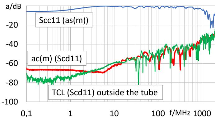
Because there is no shield in the unshielded pair, there is no near-end short circuit and no reflection. The near end wave runs back to the analyzer and can be measured there as Scd11.
