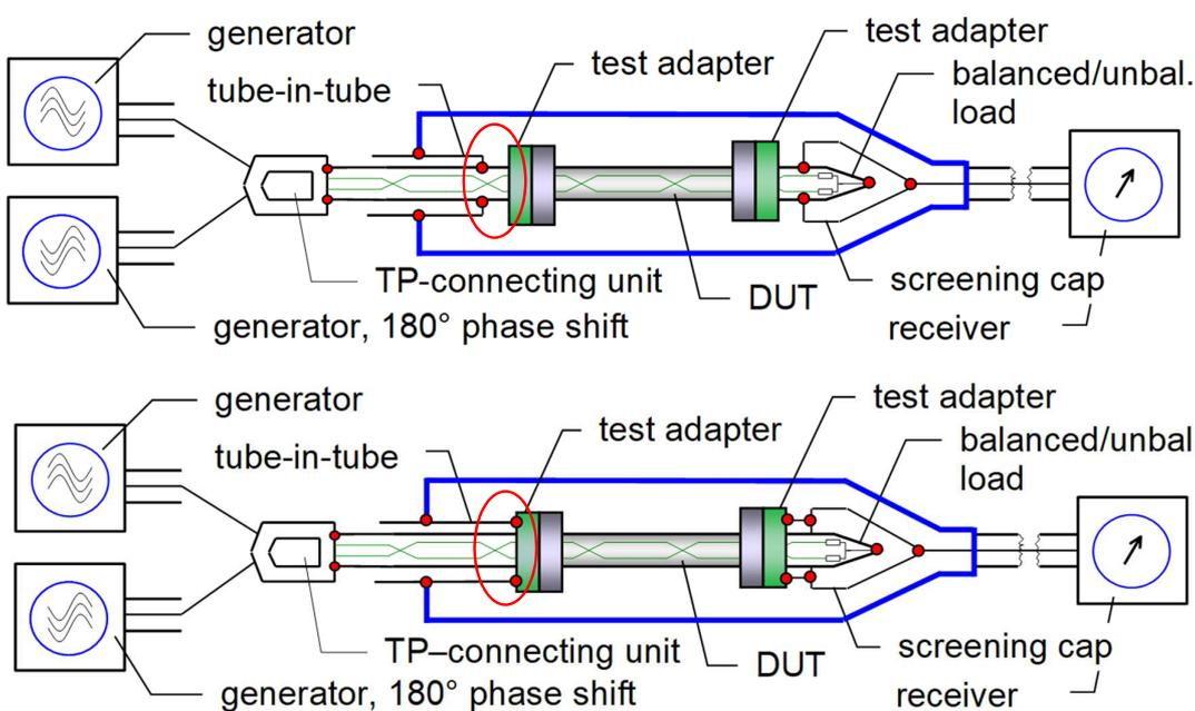
Test set-up for SPE assemblies with **tube-in-tube**.
