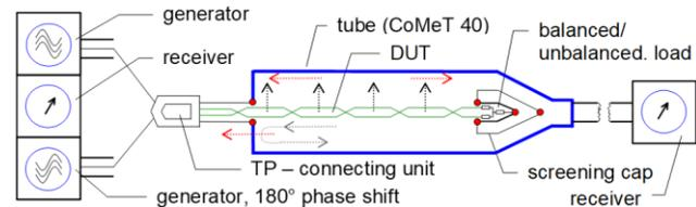
**Figure 8: Coupling attenuation of unscreened balanced cables**
