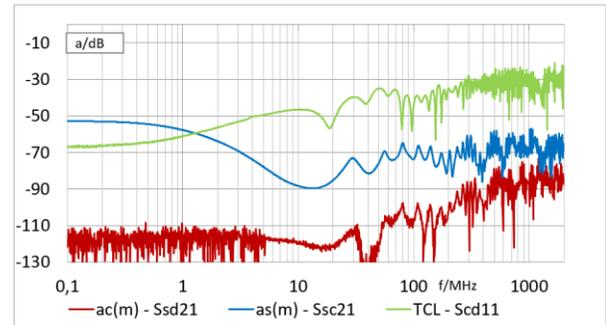
**Figure 4: Unbalance attenuation  $a_U$  (Scd11, TCL), screening attenuation  $a_s(m)$  (Ssc21) and coupling attenuation  $a_c(m)$  CA/LFCA (Ssd21) 5m SPE cable, raw values**
