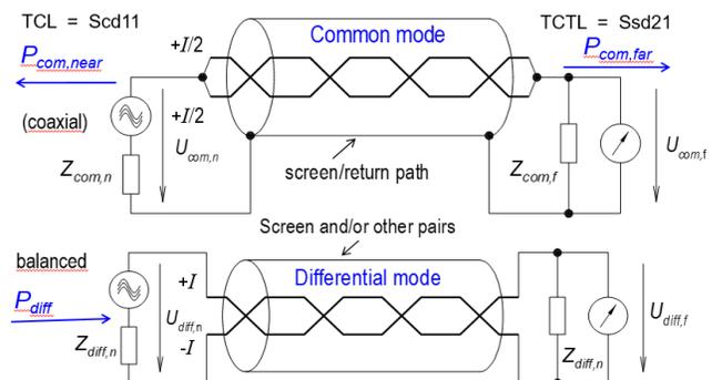
**Figure 1 - Common and differential mode of a screened twisted pair (STP)**
