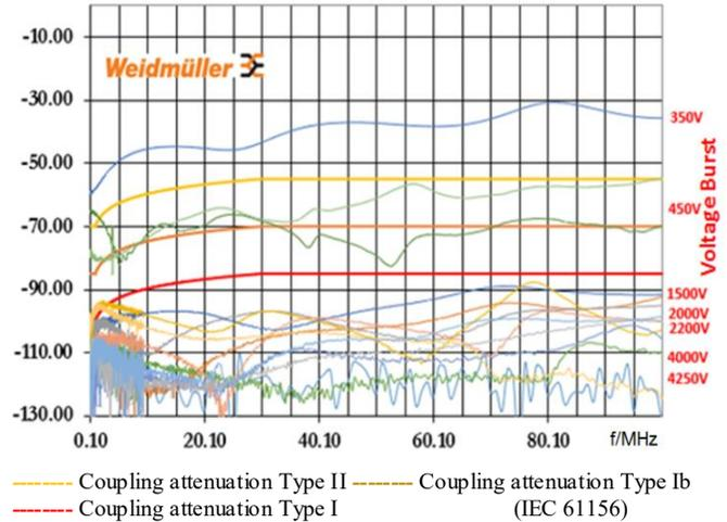
Figure 14: Correlation between Coupling attenuation and Burst test
