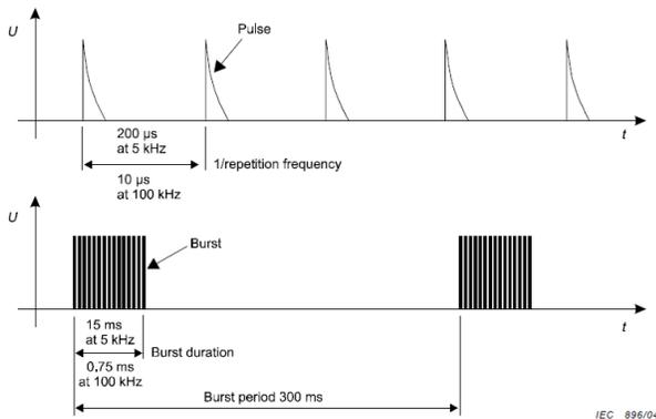
Figure 10 – Burst signal (source: IEC 61000-4-4)
