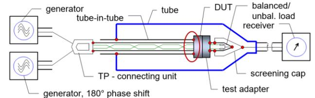
**Figure 5b: Measuring CA/LFCA of a connector with tube-in-tube with direct connection**
