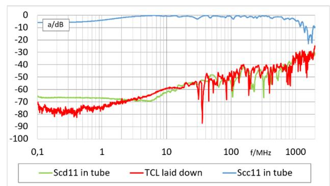
**Figure 9: LFCA/CA of an unscreened balanced cable**
