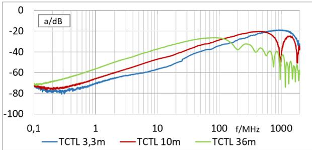
**Figure 2b: Unbalance attenuation of a shielded SPE cable at the far end (TCTL), different lengths**
