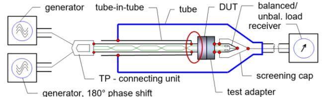
**Figure 5a: Measuring CA/LFCA of a connector with tube-in-tube with short piece of connecting cable**
