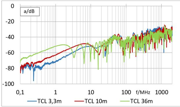
**Figure 2a: Unbalance attenuation of a shielded SPE cable at the near end (TCL), different lengths**
