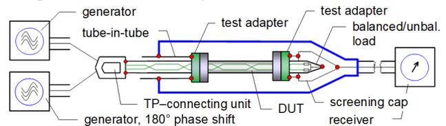
**Figure 6: Measuring the coupling attenuation  $a_c$  of a balanced assembly with tube-in-tube method according to IEC 62153-4-7 with test adapter**
