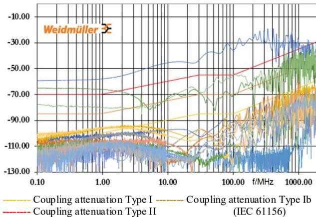
Figure 13: Coupling attenuation of different SPE cables
