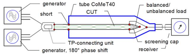
**Figure 3: Measurement of the coupling attenuation  $a_c$  of a screened balanced SPE cable with multi-port VNA and with virtual balun according to IEC 62153-4-9**
