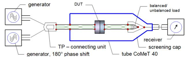
**Figure 7: Measuring of CA/LFCA (Scd21) of a pair of SPE connectors in the middle of the tube**
