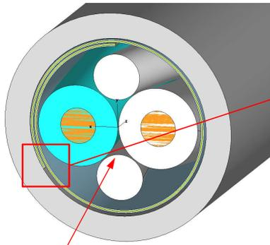
Twisted Pair cable with two filler elements and foil screen
