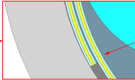
Foil shield made of Al foil with insulator on both sides. Overlap approx. 30%
