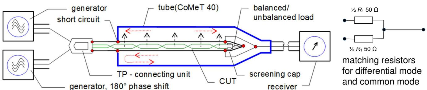
The balanced pair is fed with a 100 Ohm signal by two 50 Ohm generators with 180° phase shift (**virtual balun**). Energy couples from the “differential mode” into the “common mode” (**mode conversion**) and then from the “common mode” into the measuring tube (the outer circuit).
